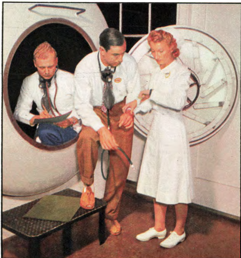
NURSE POWERS CHECKS Technician Lapworth's pulse as he emerges from a test flight in the pressure chamber. Tests show that collapse sets in unless pilots don oxygen masks (Lapworth has one around his neck) at 15,000 feet.
