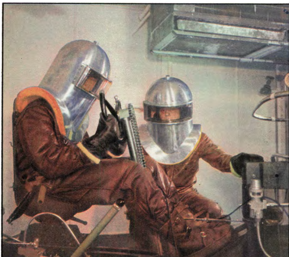
IN THE COLD ROOM, technicians test plane parts in the terrific frost met at high altitudes. Mixture of carbon dioxide and methyl
